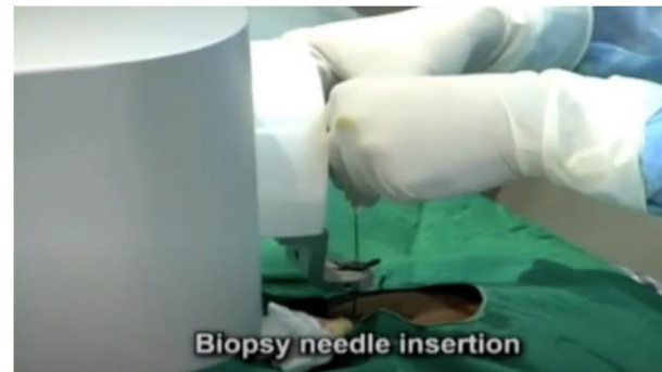
Fig. 3. Robot-assisted navigation system for computed tomography-guided percutaneous lung procedures. Needle placement via the robotic arm at the location of planned pathway.
